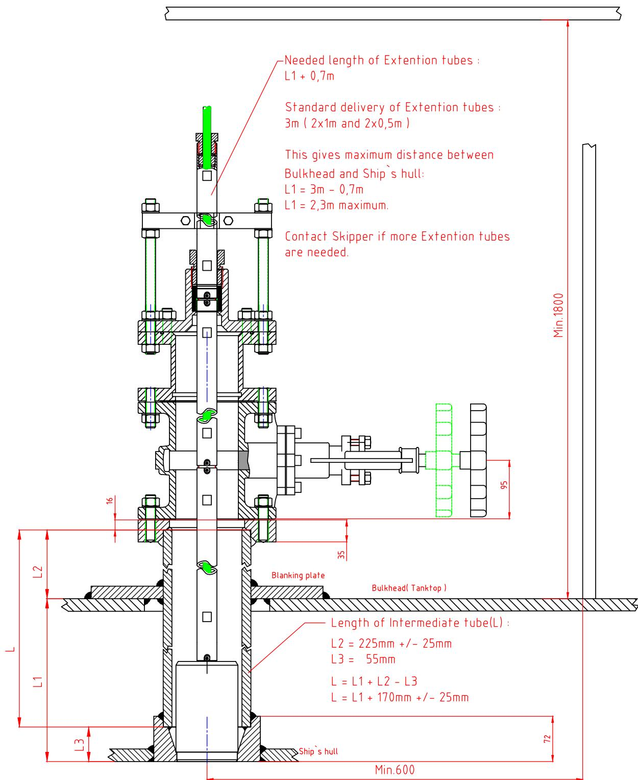
The Sea Valve should be placed in a service accessible place, large enough for installation and disassembly of the sensor unit.
